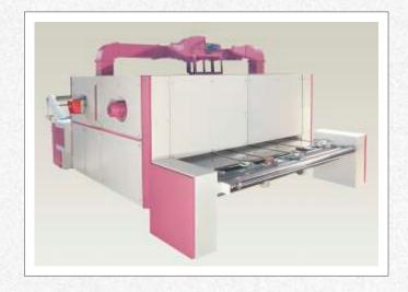
The use of the THS Heat Setting for the treatment of Cotton-Elastane / Lycra blends, as well as Synthetics and Synthetic blends, eliminates many of the problems. Heat Setting contributes significantly to the simplification of the process and therefore an appreciable reduction in processing costs.
