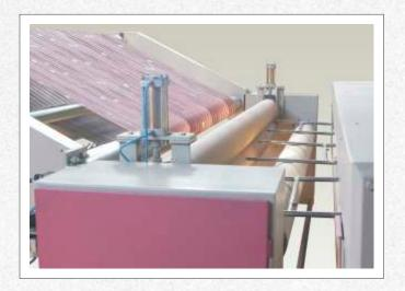
The Heat Setting machine THS is equipped with specially designed adjustable Stainless Steel Frames. Machine is equipped with Radial Blowers, one per section, a Natural Gas Burner or Thermic Fluid Heater, Nozzle Systems for uniform distribution of the re-circulating hot air and a suitable duct. The maximum temperature can be achieved upto 220°C. Machine is suitable for One, Two or Three Tubes.
