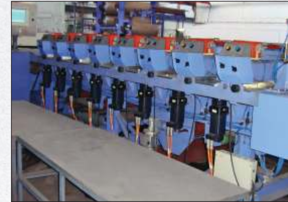
SERVO MOTOR ON EACH PRINTING POSITION
