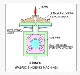
SWASTIK's specially designed gas burner has been built based on long experience and careful study aimed at overcoming such troubles and to ensure the best singeing results for a wide range of fabrics such as Cotton-Rayon-Wool and Synthetic or Blended fabrics.
