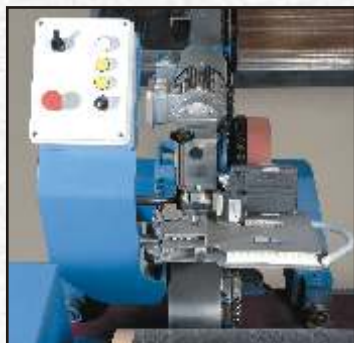
FABRIC FEEDING WITH IN-FEED DEVICE AND INFRA-RED SENSOR
